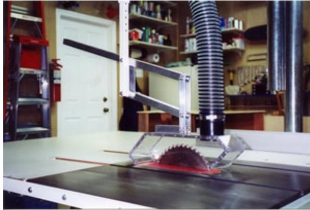
**Blade guard with the structural assembly**
