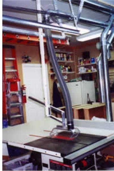
**The entire system, including the steel tubing and dust collection**
