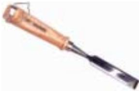
**Sandvik:** Tang chisel with a tapered beech handle and two steel ferrules. This chisel got into the test because James Krenov uses its parents and I wanted some Swedish steel. The apple fell pretty far from the tree. Though its steel and handling are good, the finish and packaging says "utility chisel". The edge is so slightly beveled that there may be clearance problems in dovetail work.
