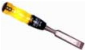
**Stanley 900:** This is the classic modern plastic handled tang chisel with a metal hammer cap on top. Its lowlights include a shaft straight from the roughing bit, heavy handling, and a blade that Stanley didn't bother to degauss. Decent steel, made in England, makes this chisel the value leader. Beginners would be well served, as might experienced
