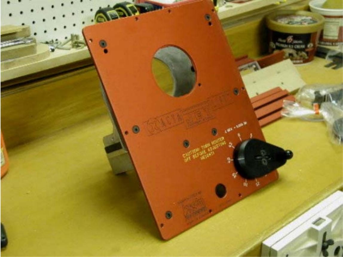
The manual has supplemental pages that made assembly pretty easy. At first glance, the plate to mount the router looks impossible to install, because of all the holes. But the instructions have clear diagrams showing the specific holes to be used for specific routers. I checked the set up for the two routers I have, the DW621 and the Bosch 1617 and they both were dead nuts on.
